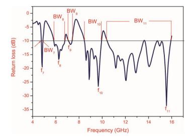
Fig. 4 Variation of return loss versus frequency of SPRMA
