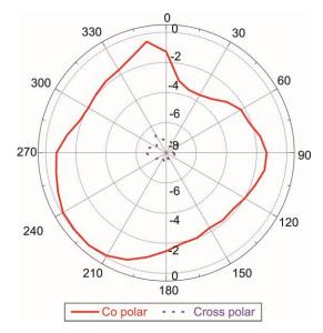
Fig. 5 Radiation pattern of PRMA measured at 4.74 GHz
