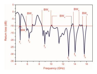
Fig. 3 Variation of return loss versus frequency of PRMA
