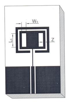
Fig. 2 Top view geometry of SPRMA
