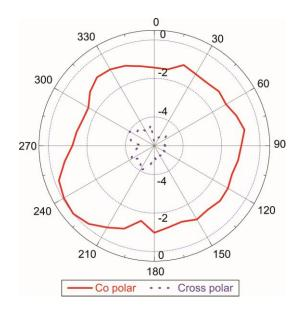
Fig. 6 Radiation pattern of SPRMA measured at 4.74 GHz
