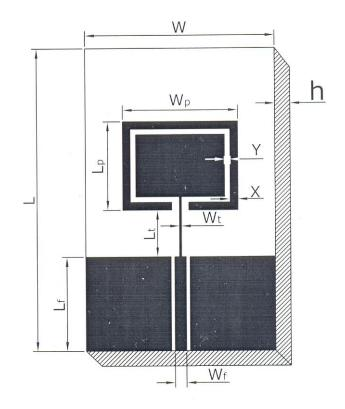
Fig. 1 Top view geometry of PRMA
